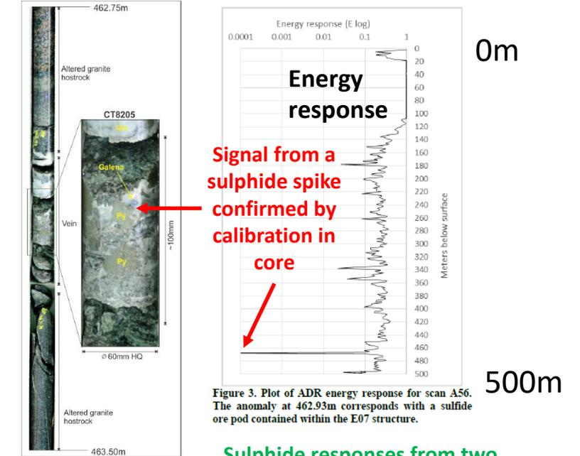
Figure 2. Diagram showing the ~100-200mm intercept in diamond drill hole CT8205 pinpointed by ADR scan A56.
