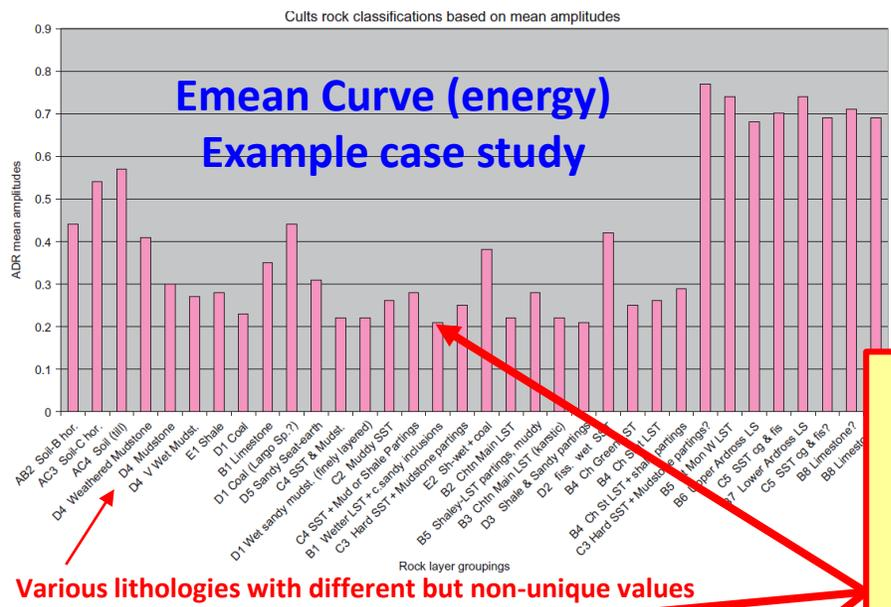
Energy, frequency, DC curves all varying as a function of lithology, but not always with *unique* values for each lithology for any one curve
