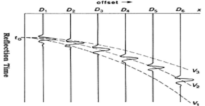
Transmitter & Receiver Normal Move Out (NMO) with increased distance
